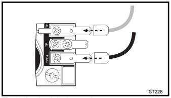
Fig. 17 Attach switch wires to valve.
